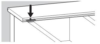
**NOTE:** The Phantom universal fastener provides a 3/16 in. side-to-side gap between each deck board and is designed to be 1-1/2 in. wide to completely cover the joist and further enhance the hidden fastener aesthetics.
